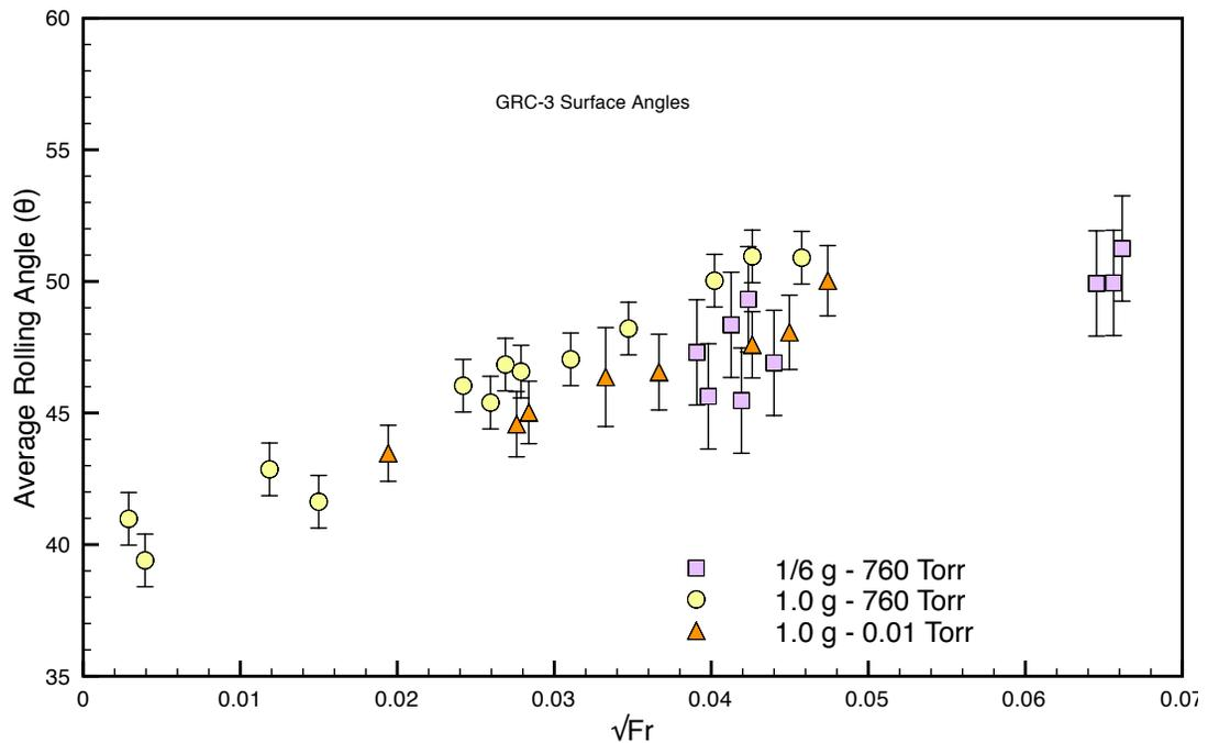
Figure 4: Measured surface angles for GRC-3. Error bars indicate variance in the measurement sets.
