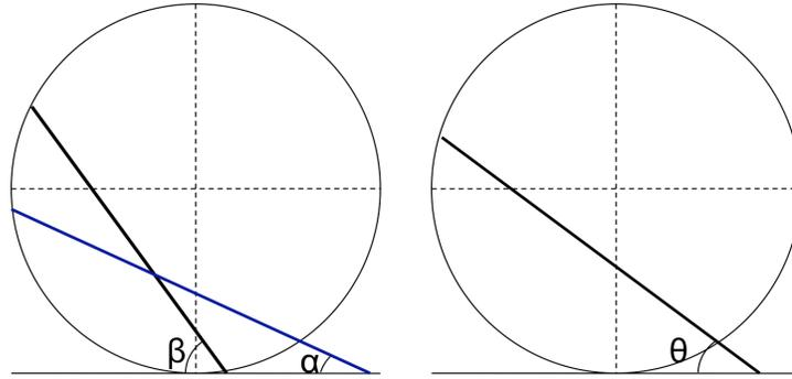
Figure 2: Surface angles measured in the the experiments. In regime 1, heap angle increases until the heap reaches the maximum stability angle  $\beta$  before collapsing to the static repose angle  $\alpha$ . In regime 2, drum rotation rates are sufficient to keep the surface flowing freely at constant repose angle  $\theta$ .
