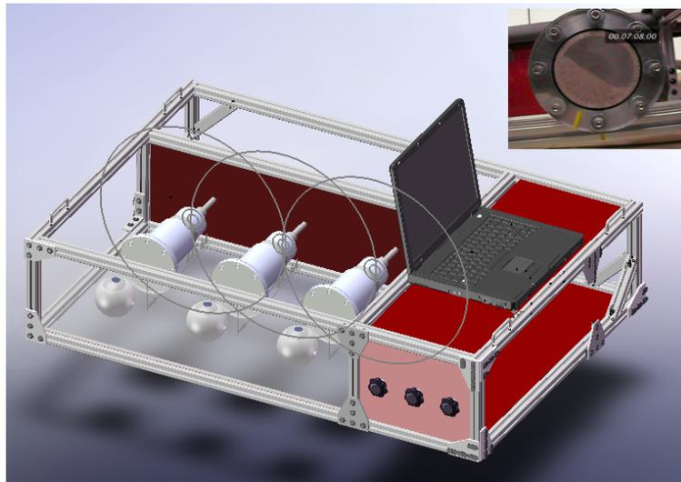
Figure 1: Experimental rig schematic and close-up of a simulant drum loaded with GRC-3 at a 30% fill. Each of the three drums has a video camera aligned with the drum view window to record simulant flow. The drums have vacuum flanged fittings and can be mounted to a diffusion pump for low pressure investigations.
