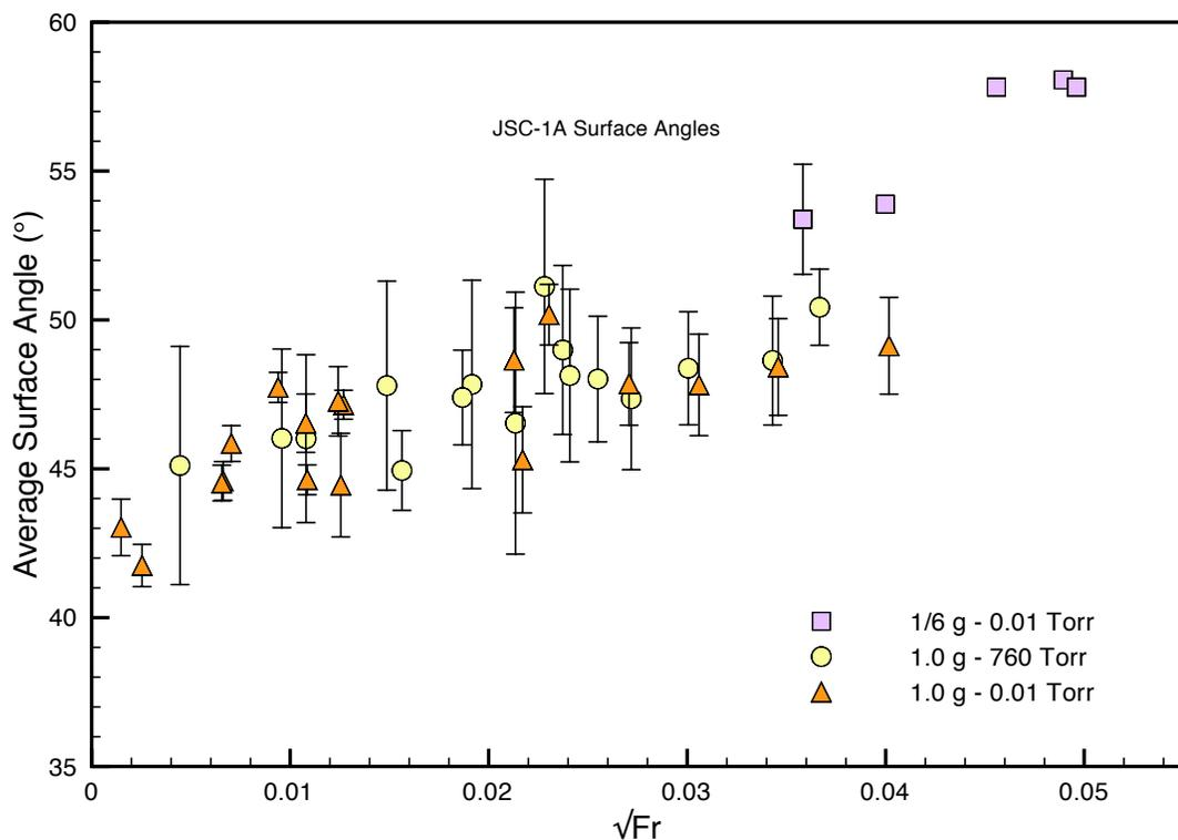
Figure 3: Measured surface angles for JSC-1A. Error bars indicate variance in the measurement sets. Uncertainty for most lunar (1/6-g) data is not available because each data point represents only one or two angle measurements.
