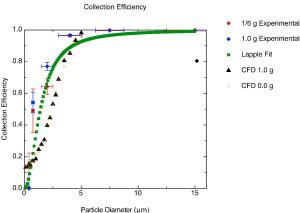
Figure 1: Experimental results (• and  $\diamond$ ), CFD results( $\blacktriangle$  and  $\times$ ), and Lapple Model predictions ( $\blacksquare$ ) for the performance of the model cyclone used in this study.
